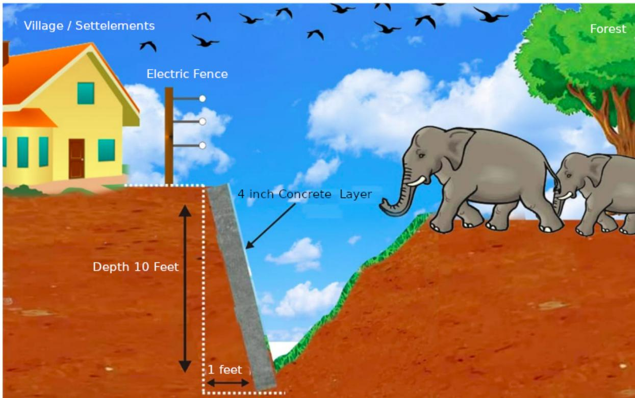
Excavate the existing trench to increase the depth. Reinforce the wall towards the village-side with concrete 4 inches thick to prevent elephants from climbing up.
